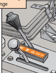
Shift the transfer shifter through neutral to the desired range. Some gear clash may occur and is normal, but you should be able to make the shift easily. Keep in mind, though, that the longer you leave the shifter in neutral, the more gear clash will occur. That's because even in neutral, engine rotation spins the transmission output shaft.
