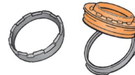
Remember to reinstall AN/PVS-14 light interference filter
