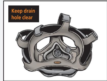
**Don't fold the mask when you put it in the carrier.** That ruins the mask. The mask goes in the carrier in the upright position with the eye lenses facing away from your body when worn in the shoulder, leg or load-bearing harness positions.
