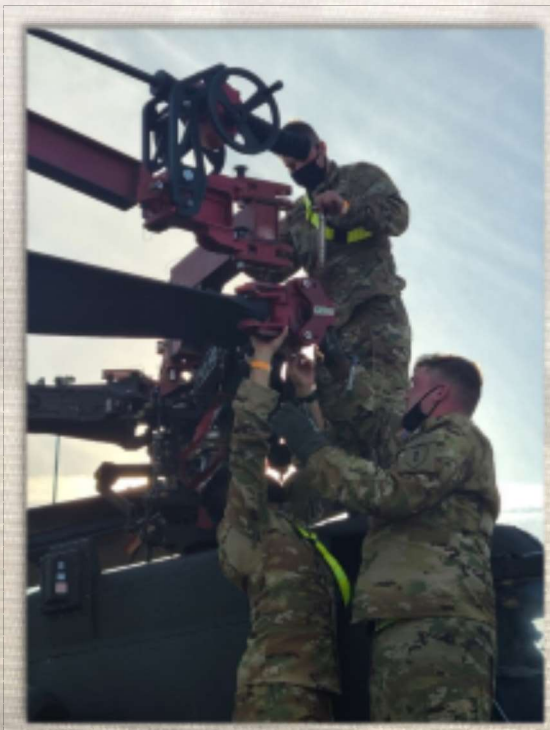
Right: SPC Harvey and PFC Daniels D Troop 2/6 CAV adjust the outer brace of the blade fold kit as they finish folding their AH-64D for transport at Hickam Field, Hawaii.
