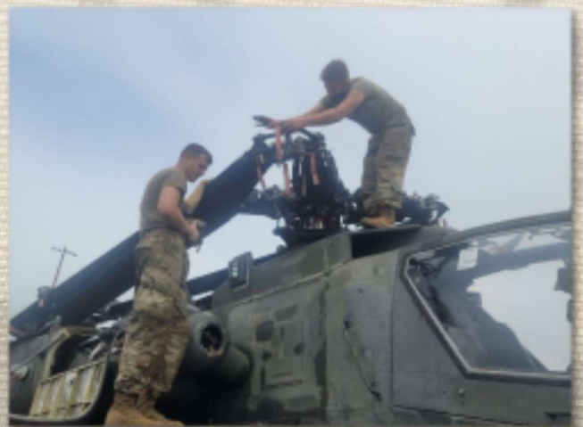
Right: SPC Harvey and PFC Daniels D Troop 2/6 CAV adjust the outer brace of the blade fold kit as they finish folding their AH-64D for transport at Hickam Field, Hawaii.
