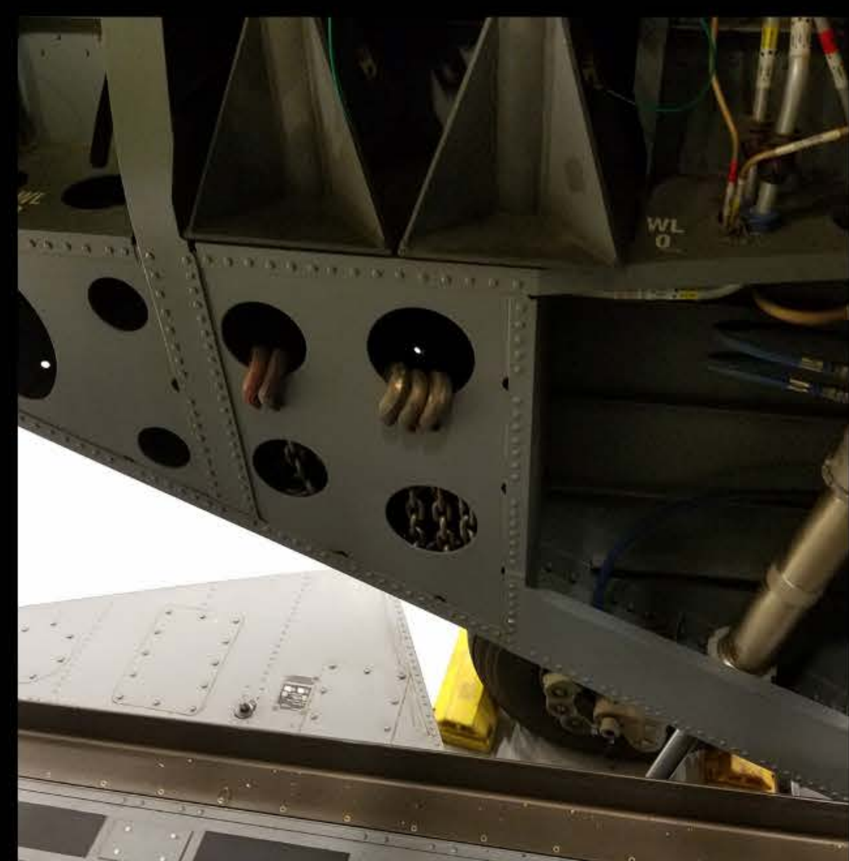
Don't store tie-down chains in canted beam area on either side of aircraft
