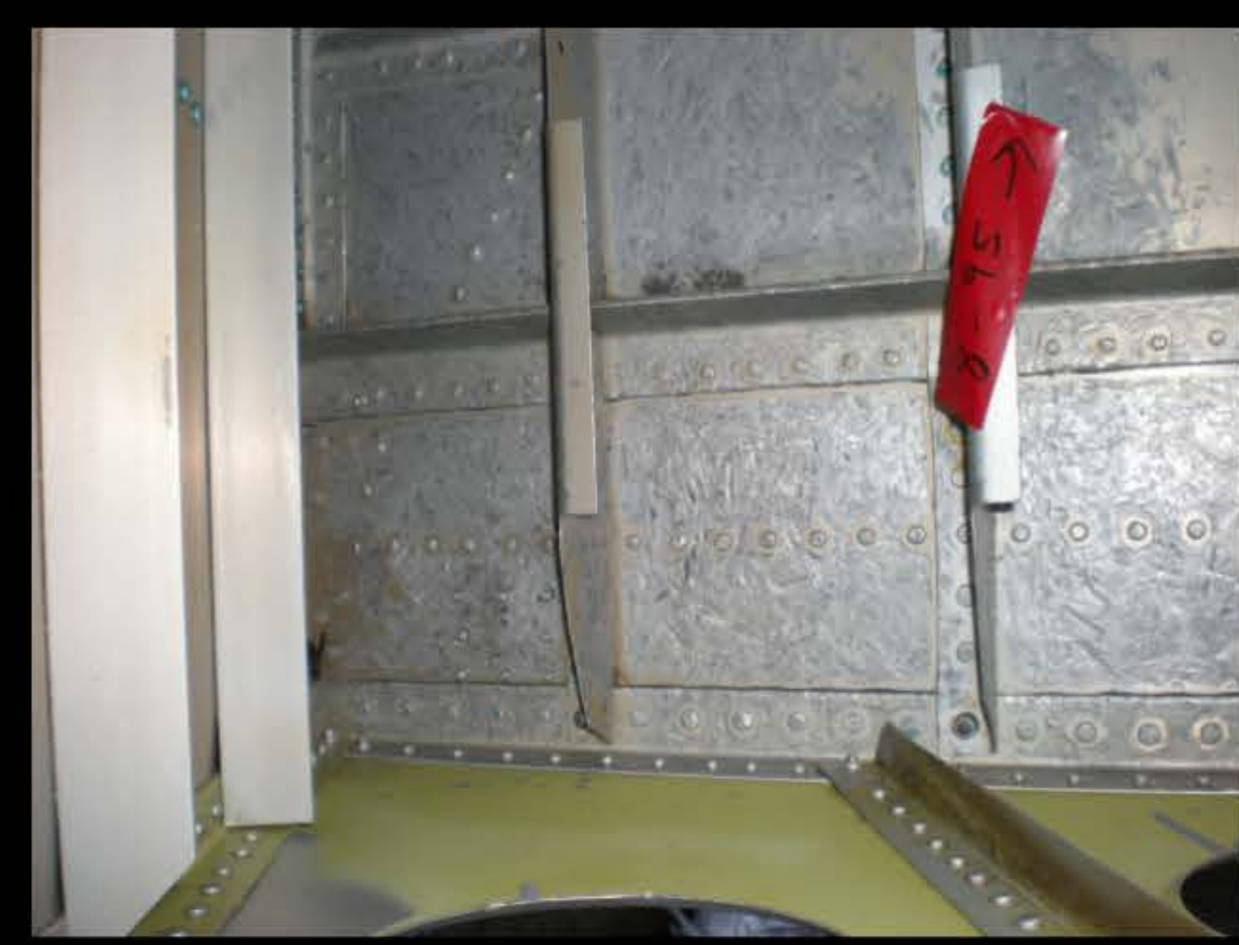
Tie-down chains can damage canted beam area on D-model
